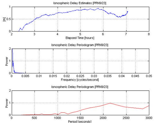
Figure 7. Example of a significant relative ionospheric delay in double-difference observations (Test 3).
