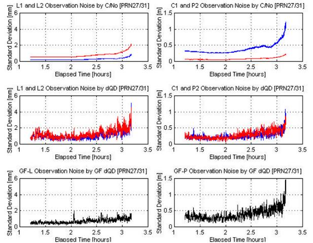
**Figure 14. Observation noise estimation (Test 1). The red line is the estimates for L1(C1) and the blue line for L2(P2).**
