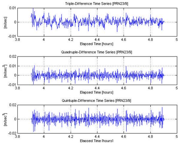
**Figure 8. Time series of the ionospheric delay change estimates (Test 3).**
