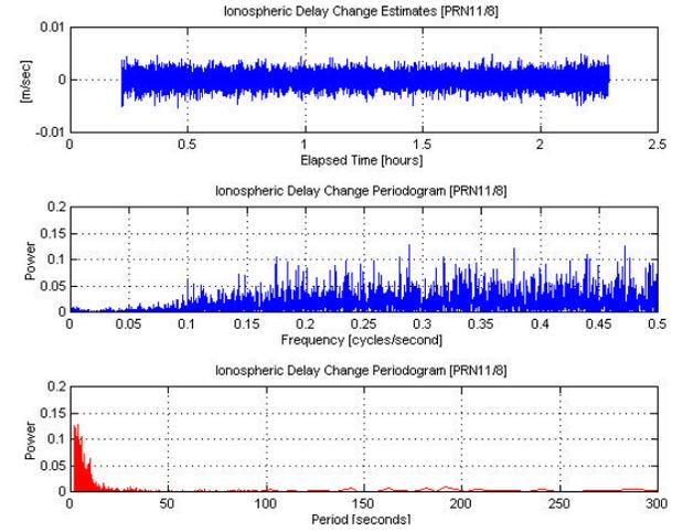
**Figure 2. Ionospheric delay change of an ideal time series and its periodogram (Test 1).**
