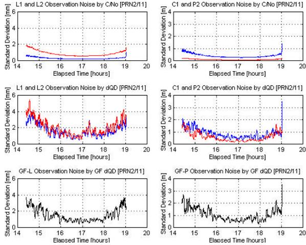
**Figure 15. Observation noise estimation (Test 3).** The red line is the estimates for L1(C1) and the blue line for L2(P2)
