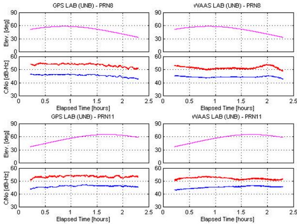
**Figure 1. Elevation angle and  $C/N_0$  for a weak multipath situation (Test 1). The red line is the  $C/N_0$  for L1(C1) and the blue line for L2(P2).**
