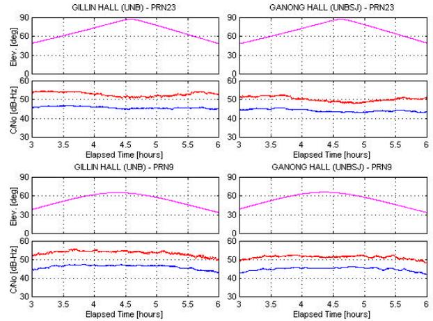
Figure 6. Elevation angle and  $C/N_0$  for long-baseline weak multipath case (Test 3). The red line is the  $C/N_0$  for L1(C1) and the blue line for L2(P2).
