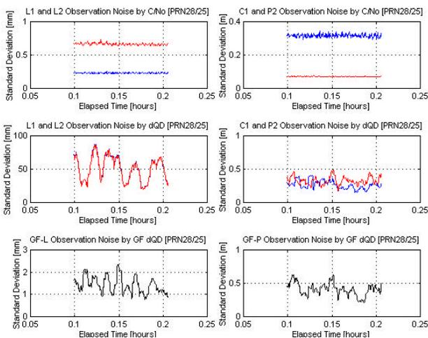
**Figure 16. Observation noise estimation (Test 2).** The red line is the estimates for L1(C1) and the blue line for L2(P2)
