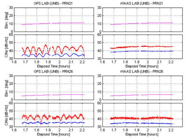
**Figure 3. Elevation angle and  $C/N_0$  for a strong multipath situation (Test 1). The red line is the  $C/N_0$  for L1(C1) and the blue line for L2(P2).**
