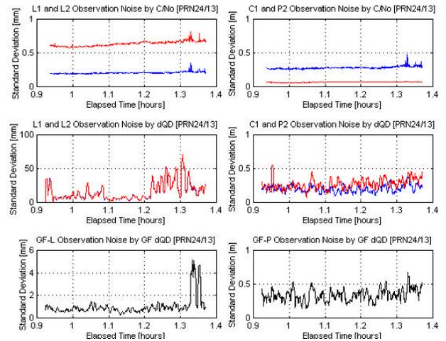
**Figure 17. Observation noise estimation (Test 4).** The red line is the estimates for L1(C1) and the blue line for L2(P2)
