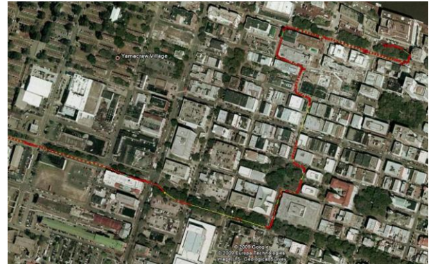
Figure 4: Position solutions in downtown Savannah from single point positioning with GPS+GIOVE (imagery courtesy of Google)
