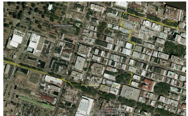
Figure 5: Position solutions in downtown Savannah from single point positioning with GPS only (imagery courtesy of Google)
