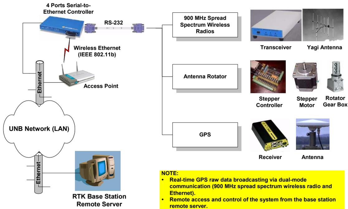
Figure 5: UNB RTK base station system components.
