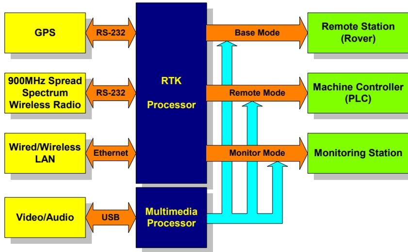
Figure 6: UNB RTK software block diagram.
