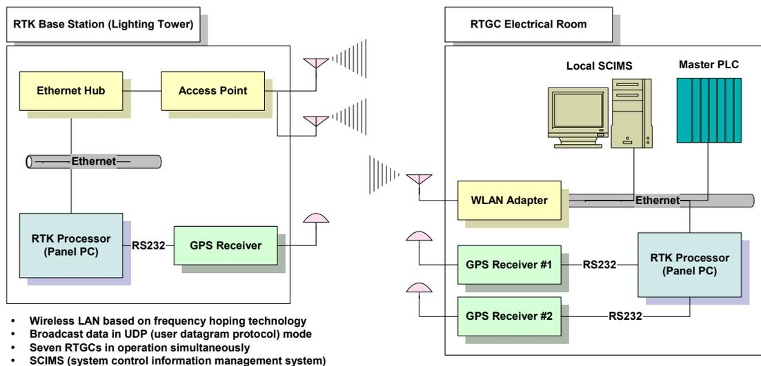
Figure 3: Sketch of the RTGC auto-steering system based on an ad hoc network using WLAN.
