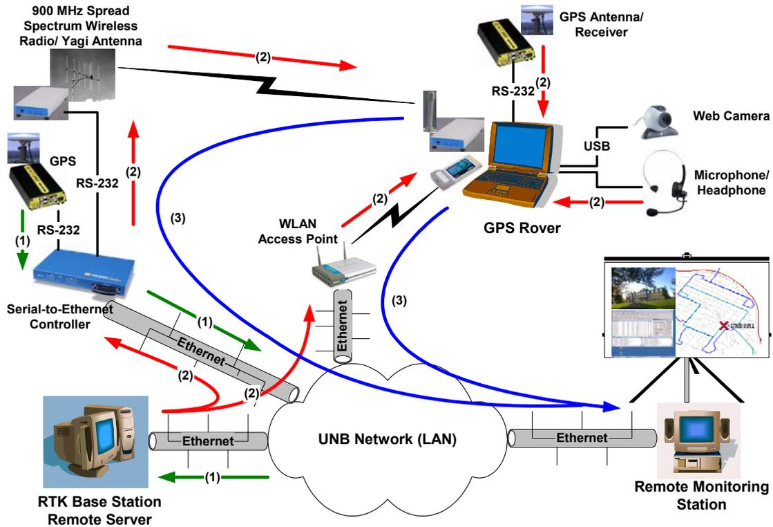
Figure 8: UNB RTK system configuration for Geo-spatial fusion demonstration.
