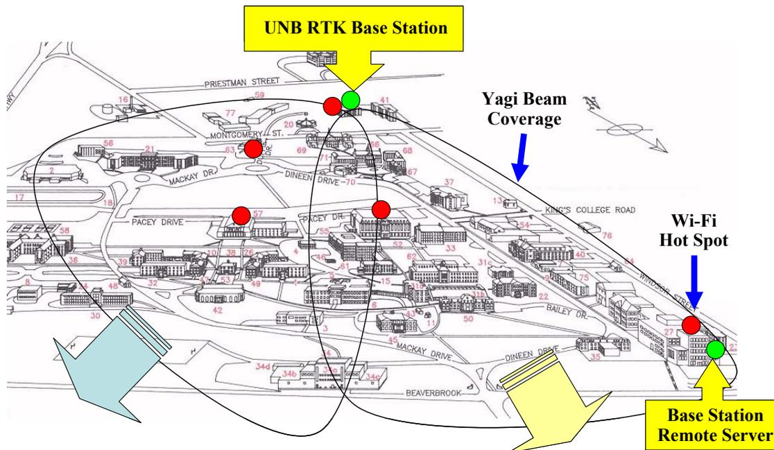
Figure 4: UNB RTK base station and broadband signal coverage.
