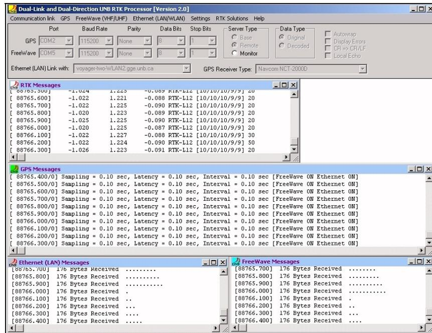
Figure 7: UNB RTK software operating in the remote mode.
