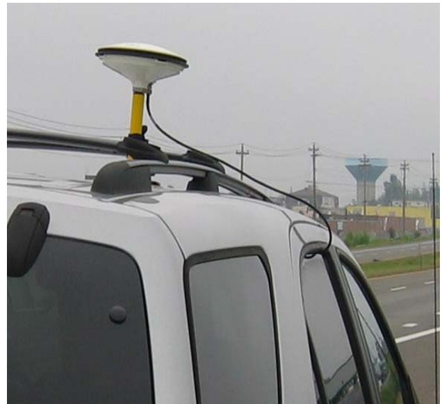
Figure 9: Setup of a NovAtel antenna on the top of the vehicle, for the kinematic test.
