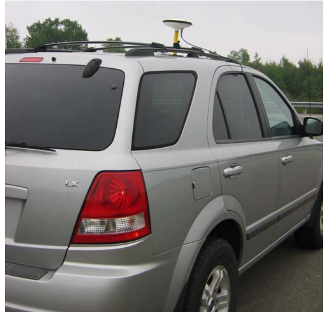
Figure 1: Platform for the kinematic test.
