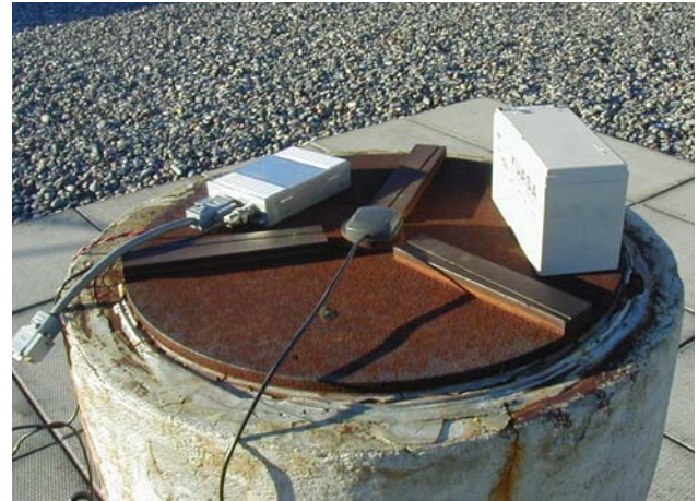
Figure 6: Components of the low-cost GPS receiver used in the static test, in a multipath environment.
