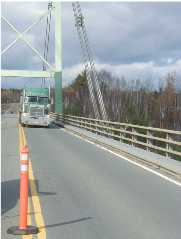
FIGURE 9 – Design truck with 50 ton paper load (information got in Paper Manufactory - Pulp Mil)
