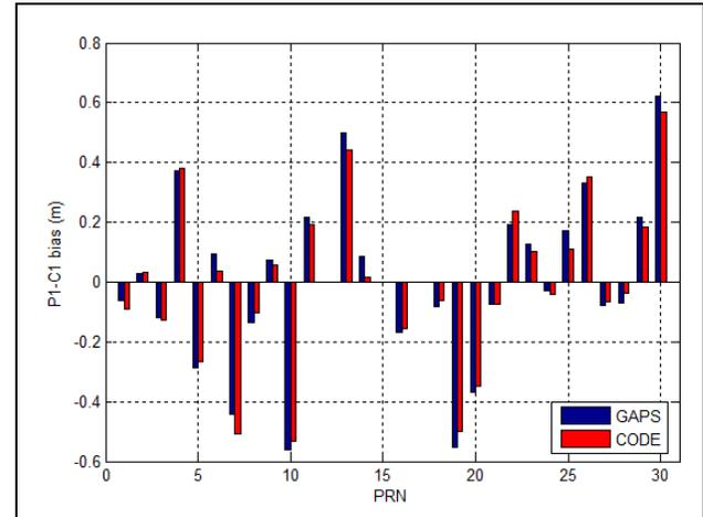
Figure 2. Comparison of satellite differential P1-C1 biases determined by CODE and with GAPS.
