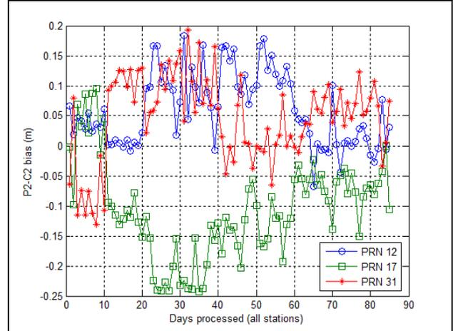
Figure 4. Results of the P2-C2 satellite bias determination for several days and stations.
