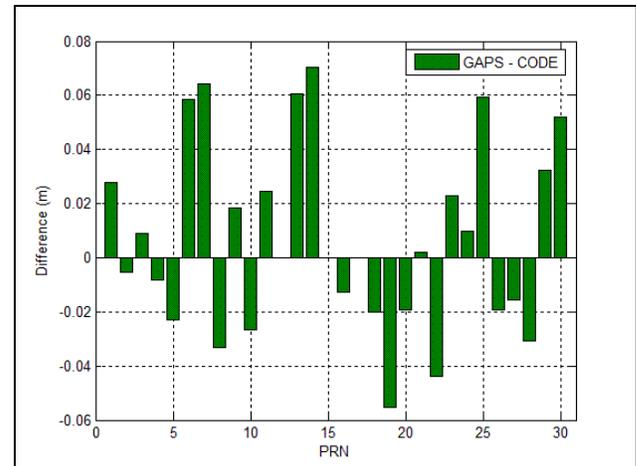
Figure 3. Differences of the satellite differential P1-C1 biases determined by CODE and with GAPS.
