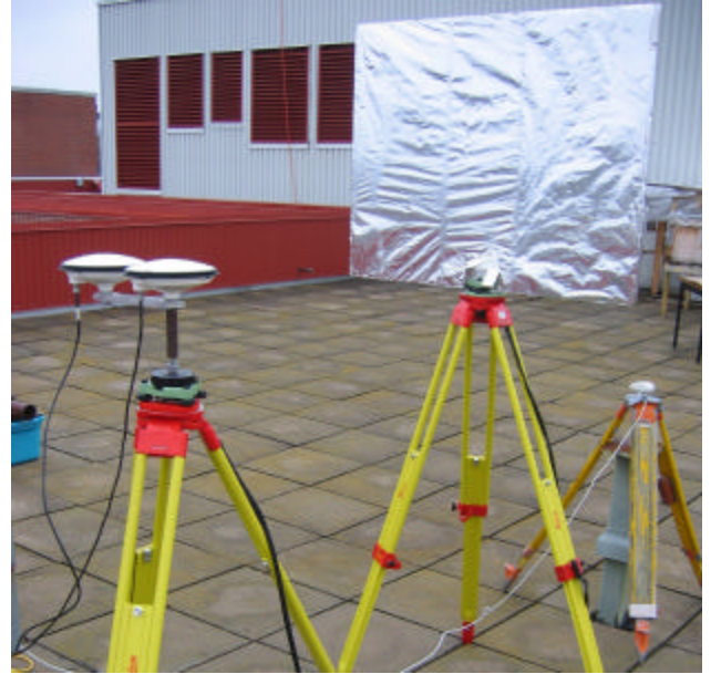
Figure 2: Scenario for the multipath profile estimation, with a strong nearby reflector and two antennas (static and mobile).
