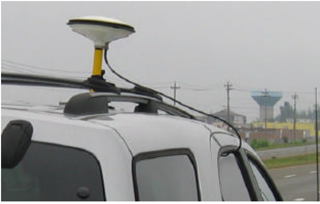
Figure 9 Setup of a NovAtel antenna on the top of a vehicle, for a kinematic test.
