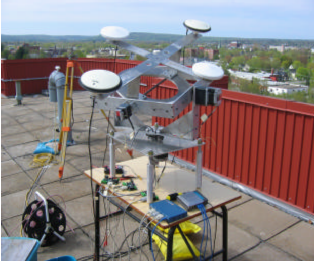
Figure 3: Scenario for the multipath profile estimation, with a motion table.
