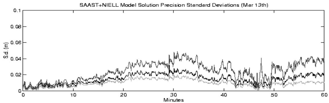
**Figure 4.** Precision of solutions (standard deviations of height, northings and eastings respectively descending the y axes).
