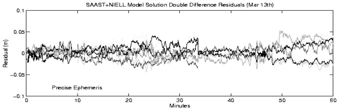
**Figure 3.** L1 Carrier Phase Double Difference Residuals (Precise Orbits).
