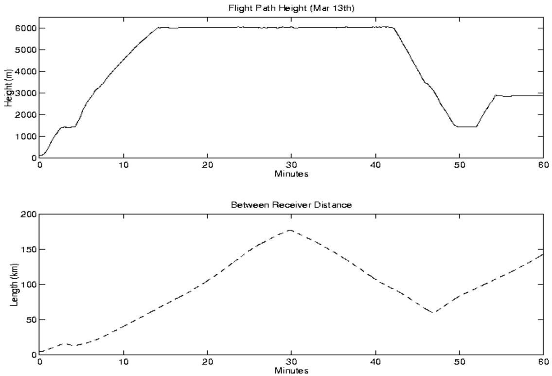
**Figure 2.** (a) Height of airplane. (b) Distance from reference receiver.
