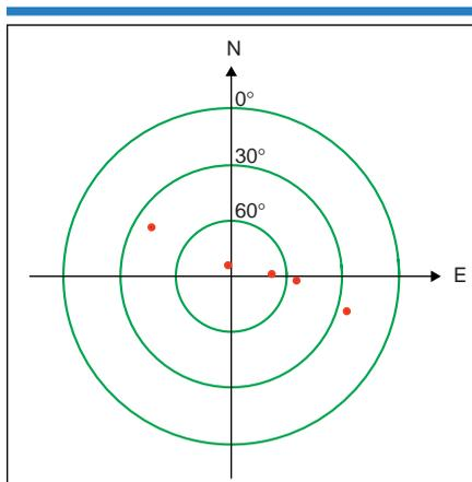
**Figure 4.** The spike in the DOP values in Figure 3 is caused by the almost perfect alignment of the five satellites above the elevation mask angle.
