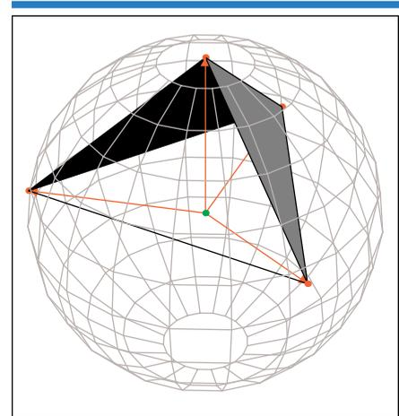
**Figure 2.** If only four GPS satellites are observed, the tips of the receiver–satellite unit vectors form a tetrahedron circumscribed by a unit sphere. Two faces of the tetrahedron — formed by one satellite at the zenith and three at a 10-degree elevation angle, equally spaced in azimuth — are shaded in this figure. The tetrahedron’s volume is highly correlated with GDOP. Maximizing the volume tends to minimize GDOP.
