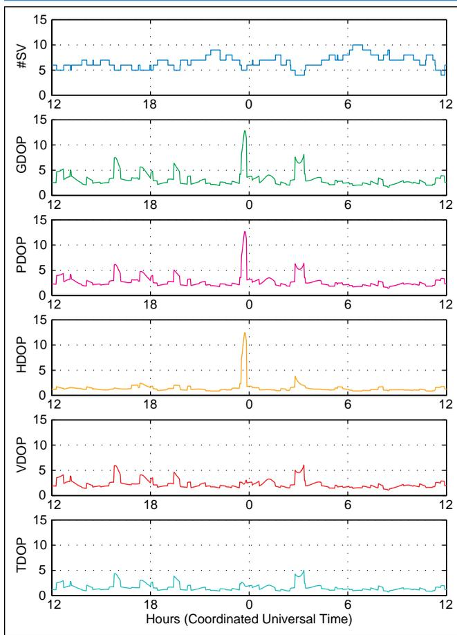
**Figure 3.** DOP values at Fredericton, New Brunswick, Canada, — computed from broadcast satellite ephemerides using a 15-degree elevation mask angle — are sufficiently small except just before 0000 hours when HDOP, PDOP, and GDOP increase to more than 12 (#SV represents the number of visible satellites [space vehicles]).
