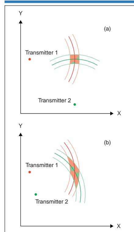
**Figure 1.** In any ranging system, receiver-transmitter geometry influences position precision. In this figure, the uncertainty in the receiver's position is indicated by the patterned areas. In (a), the position uncertainty is small (low dilution of precision). In (b), transmitter 2 is moved closer to transmitter 1, and, although the measurement uncertainty is the same, the position uncertainty is considerably larger (high dilution of precision).
