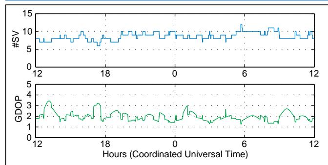
**Figure 5.** Lowering the elevation mask angle to 5 degrees removes the spikes just before 0000 hours in the DOPs of Figure 3. Now, the GDOP has an average value of about two and never exceeds 3.5 (#SV represents the number of visible satellites [space vehicles]).
