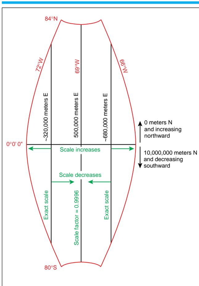
Figure 2. UTM zone 19 extends from 66 degrees to 72 degrees west longitude. As with all UTM zones, the scale factor is 0.9996 on the central meridian and true (unity) on two slightly curved lines approximately 180 kilometers to either side. The shape of the zone has been exaggerated for clarity.
