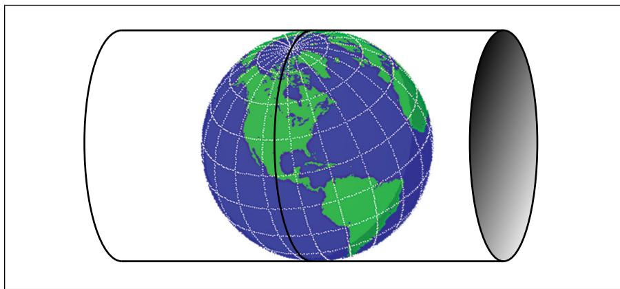
Figure 1. The transverse Mercator projection is developed on a cylinder tangent to the ellipsoid along a central meridian. The cylinder is then opened and flattened.
