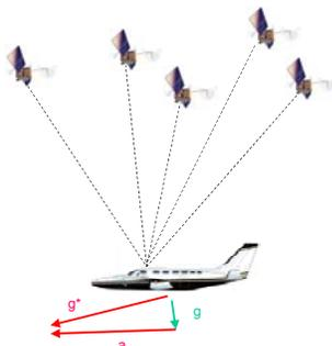
$g^*$  Total acceleration measured by accelerometers. Total acceleration is composed of:  $g$  - the earth's gravity field and  $a$  - acceleration due to the motion of the aircraft derived at a point in the aircraft from GPS position estimates.
