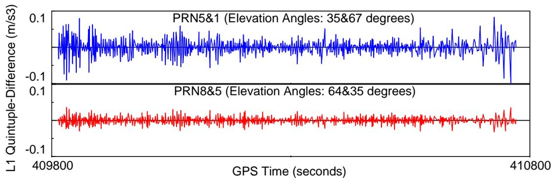
Figure 2. Observation noise modeling using Quintuple-difference time series.
