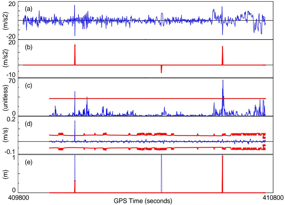
Figure 1. Example of cycle-slip detection and identification procedures (PRN15&30): (a) L1 Quadruple-difference time series; (b) Cycle-slip candidates detected by spikes; (c) Cycle-slip candidates detected by the Kalman filter prediction residuals (95% confidence level); (d) Cycle-slip candidates detected by the ionospheric delay estimates (95% confidence level); and (e) Masking results (cycle-slip identification).
