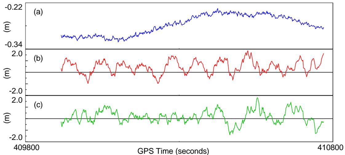
Figure 3. Kalman filter estimates (PRN9&8): (a) Ionospheric-delay; (b) Multipath in C/A pseudoranges; and (c) Multipath in P2 pseudoranges.
