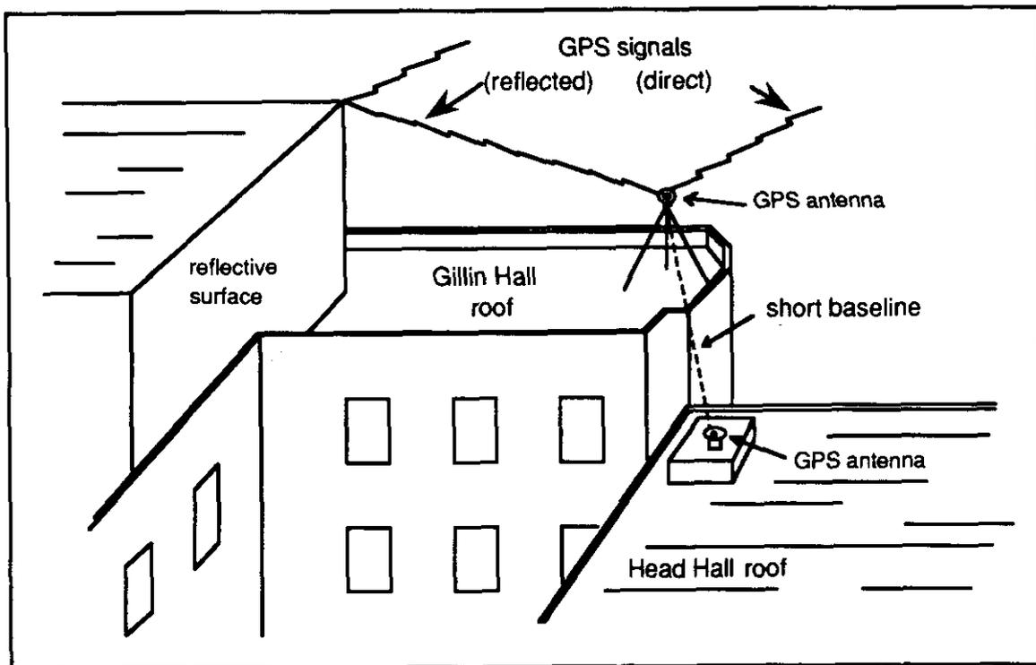
Figure 1.1 Experiment setup showing GPS signals.
