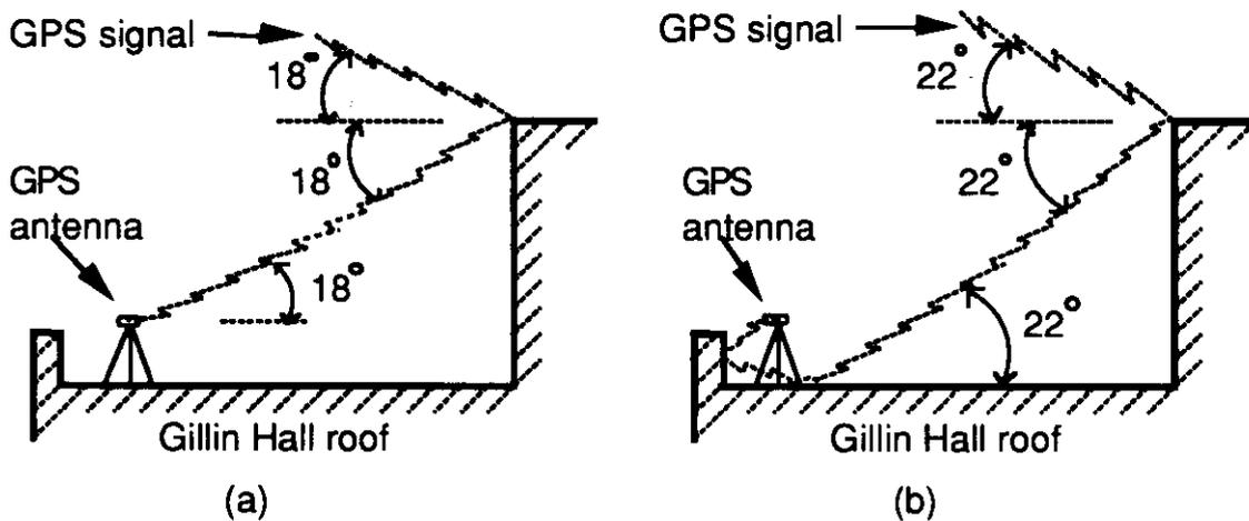
Figure 4.7 Signal reflections: Single (a), Multiple (b).
