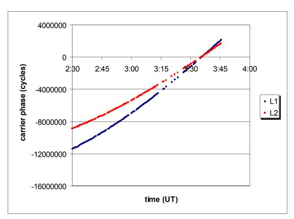
Note that there is no evidence of cycle slippage, despite the fact that the NRCan produced RINEX files do not contain data for this satellite at certain epochs. This suggests that the receiver did indeed continue to track this satellite (i.e. no "loss of lock" at the hardware level), and that the data gaps are a function of later data processing.
