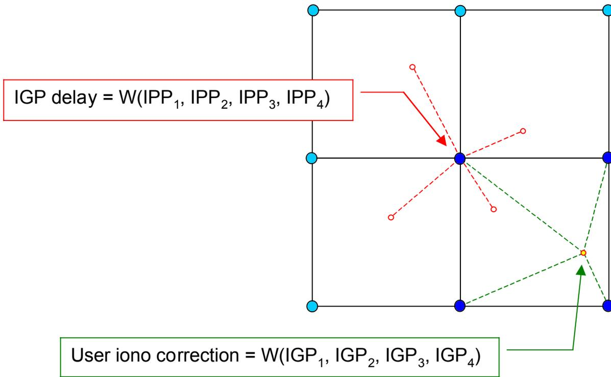
corrected pseudorange = measured pseudorange – (user iono correction \* mapping function)
