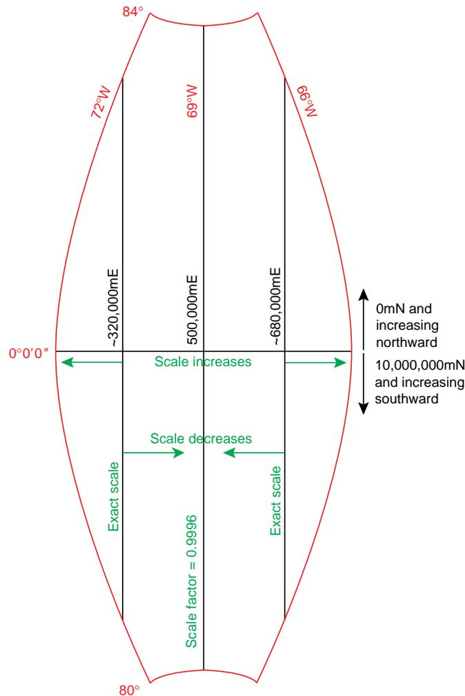
UTM zone 19 extends from  $86^\circ$  to  $72^\circ$  west longitude. As with all UTM zones, the scale factor is 0.9996 on the central meridian and true (unity) on two slightly curved lines approximately 180 km to either side. The shape of the zone has been exaggerated for clarity.
