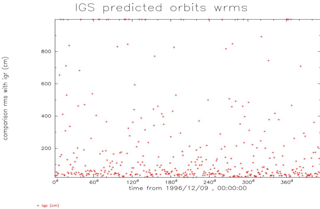
**Fig. 7 Comparison weighted rms of predicted orbits with respect to rapid orbits**
