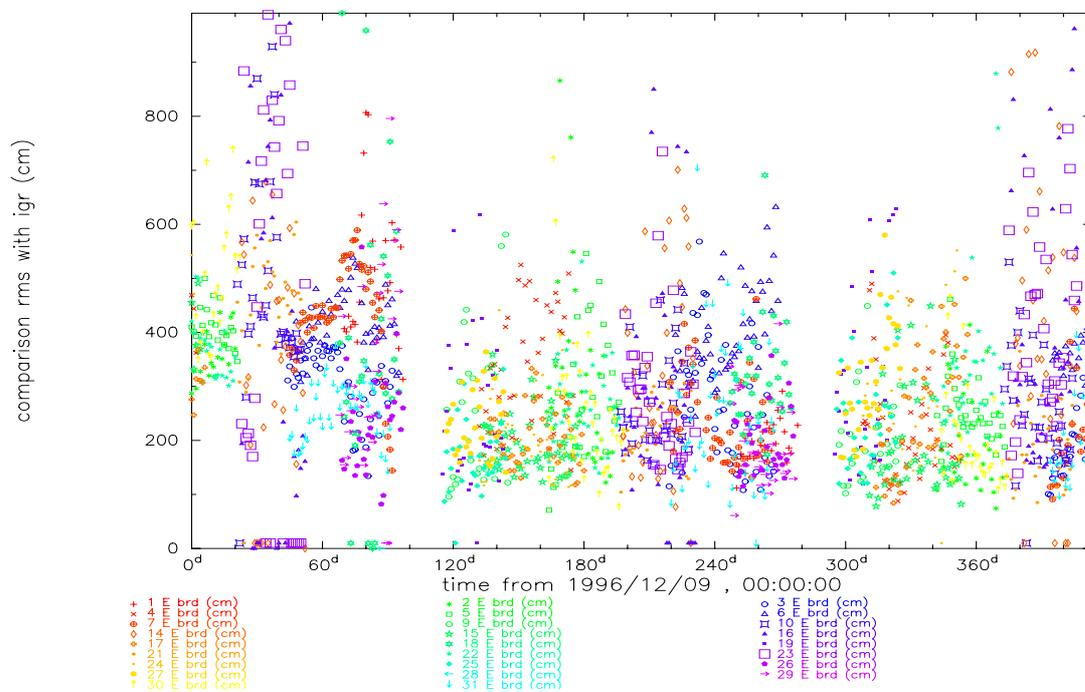
**Fig. 11 Comparison rms of broadcast orbits with respect to rapid orbits for eclipsing satellites**
