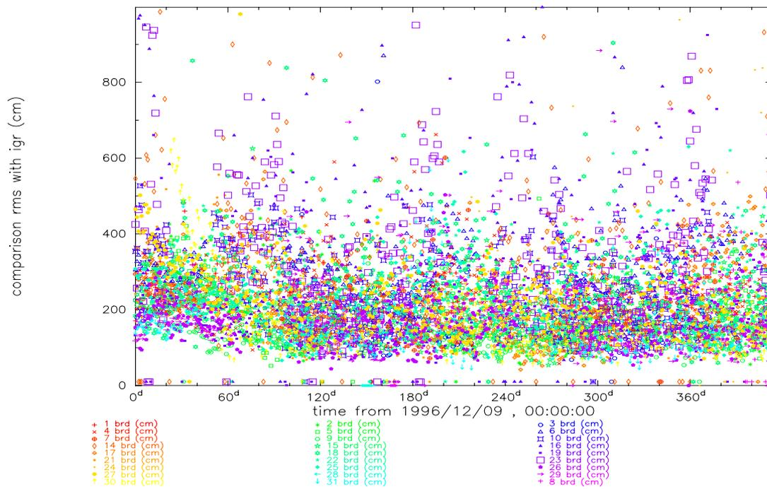
**Fig. 10 Comparison rms of broadcast orbits with respect to rapid orbits for non-eclipsing satellites**
