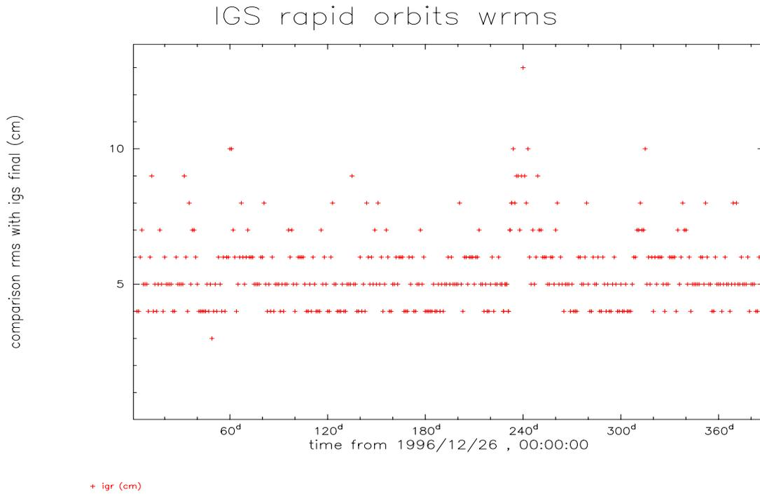
**Fig. 6 Comparison weighted rms of rapid orbits with respect to final orbits**
